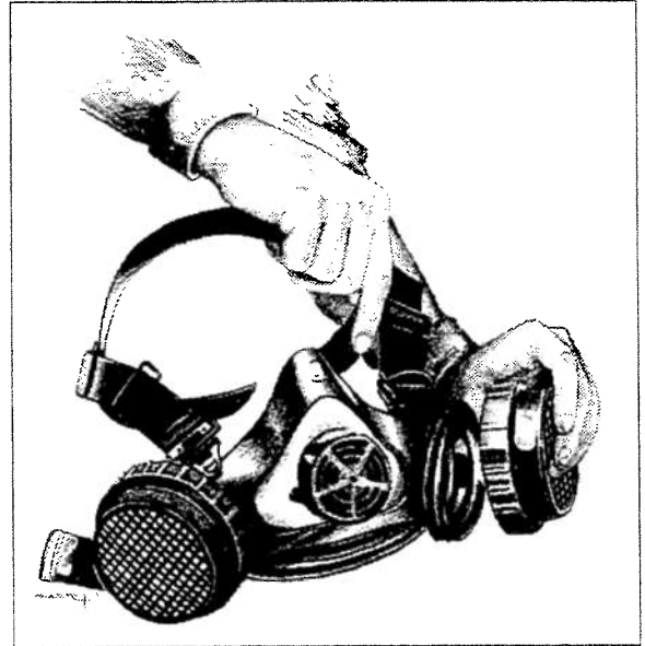
Change cartridges whenever your company's safety program recommends it. Use the right cartridge for the hazards you face and do pressure tests after replacing cartridges or filters.
